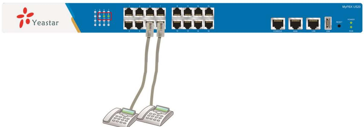
Figure 3-5 Connection of FXS ports and Status LED
