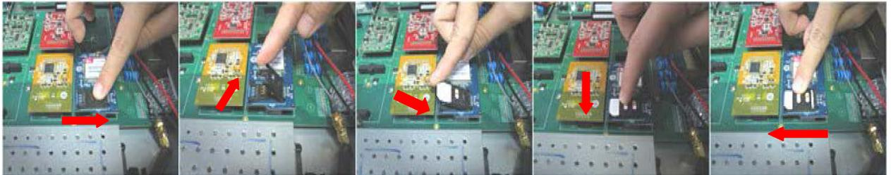
Figure 3-2 Inserting the SIM Card
