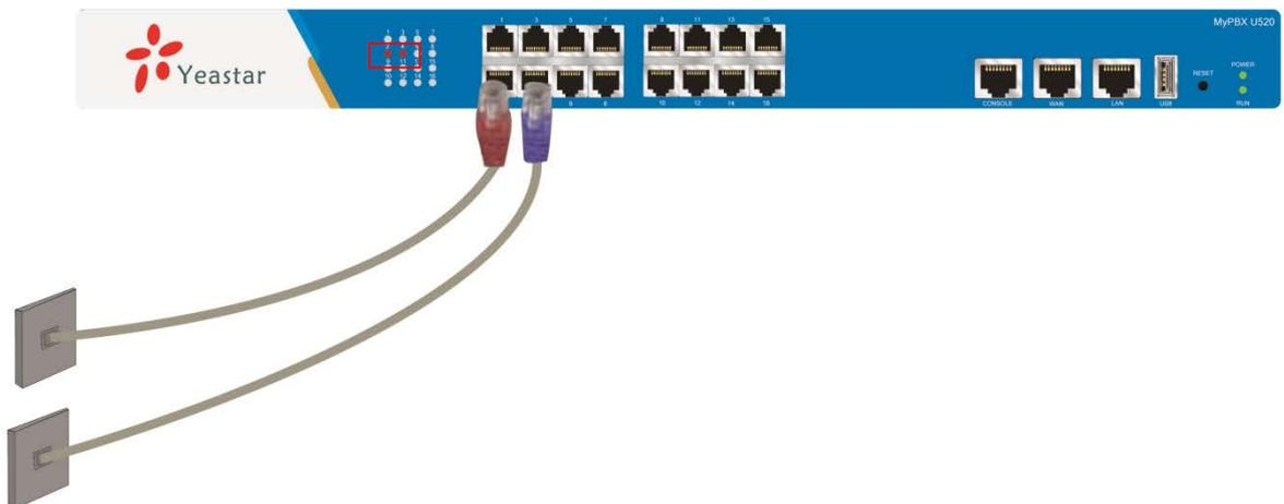
Figure 3-1 Connection of FXO ports and status LED
