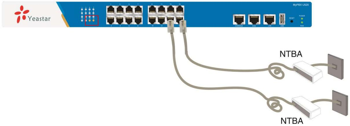
Figure 3-4 Connection of BRI ports and Status LED
